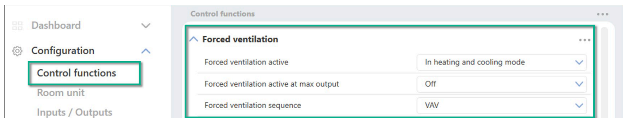
Figure 2-36 Forced ventilation configuration settings in Application tool.
